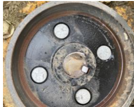
Loose Castle Nut Damage
