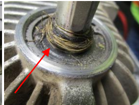
Debris wrapped on shaft
