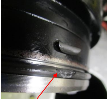
Section Seal Leak
