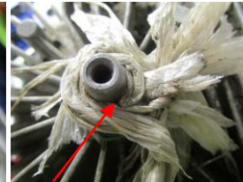
Debris wrapped on shaft
