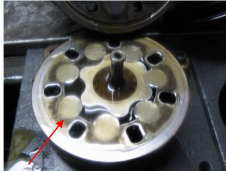
Thermal Failure to Rotor Set
