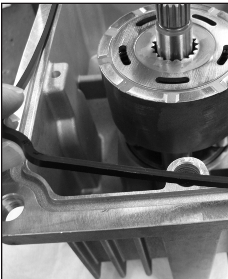
Place housing seal into groove
