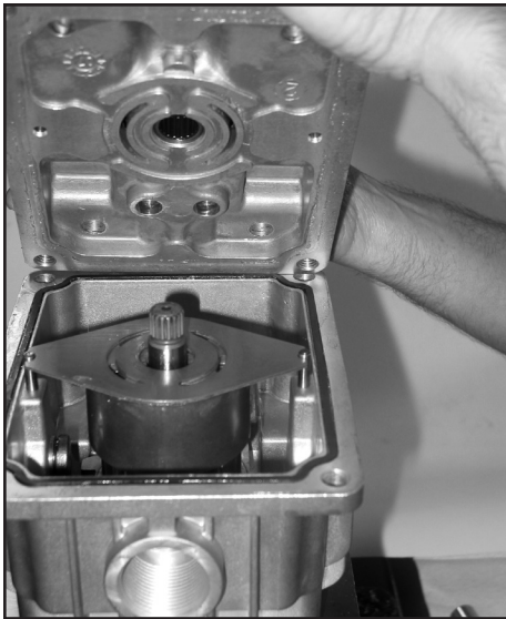
Align center block to front housing
