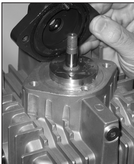
Removal of charge cover
