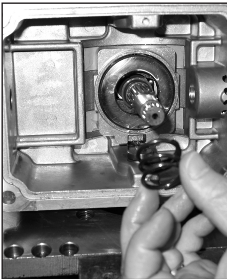
Install central spring
