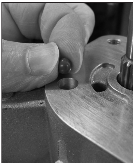
Install charge relief ball
