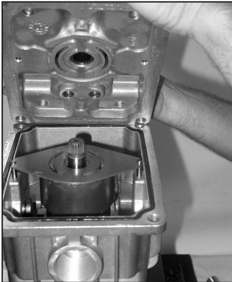
Remove center block and rear housing
