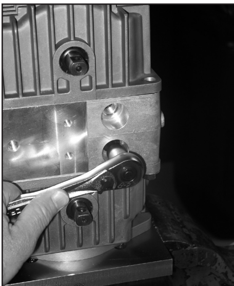
Check /shock valve removal
