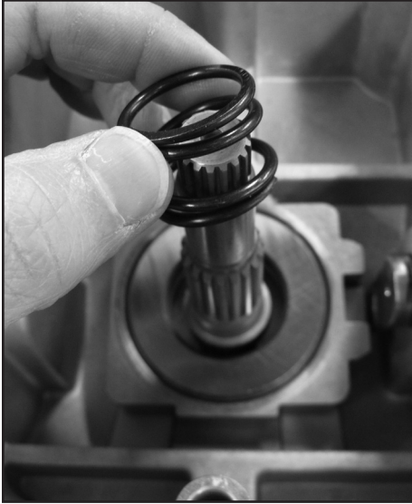
Install central spring into rear housing
