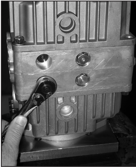
Check /shock valve removal
