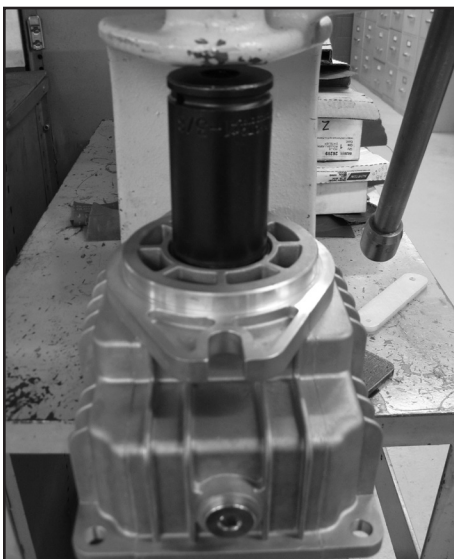
Press shaft seal into place
