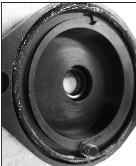
Install o-ring and spring in charge cover
