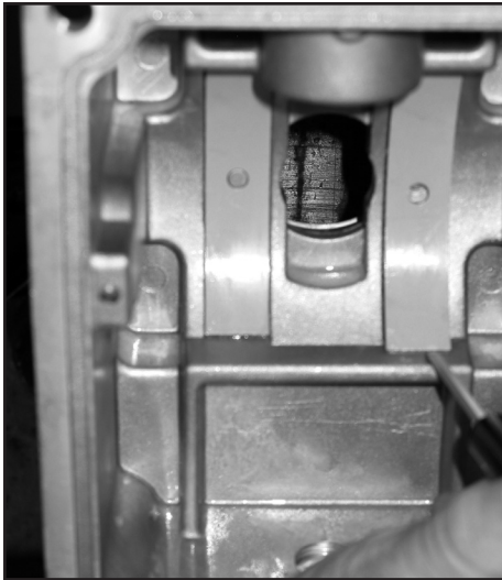
Inspection of cradle bearing
