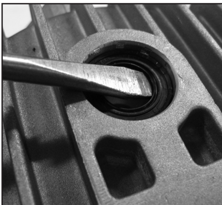
Trunnion seal removal
