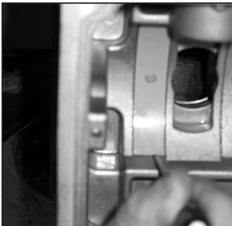
Removal of cradle bearings
