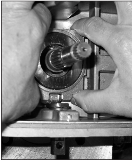
Install swash block/thrust bearing assembly
