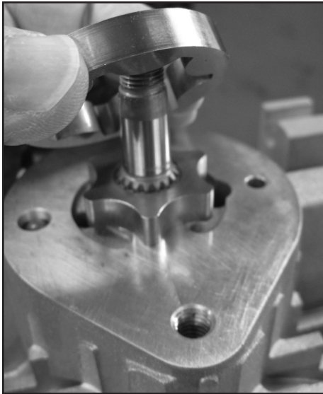
Install charge rotor set
