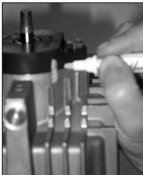
Mark charge pump cover to housing
