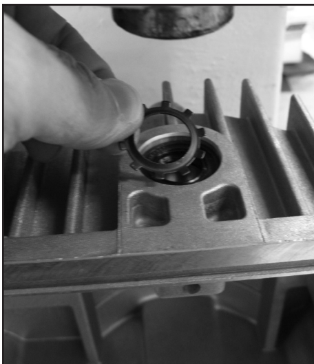
Press in seal retainers
