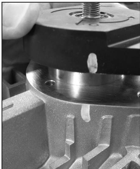
Align charge cover with marks
