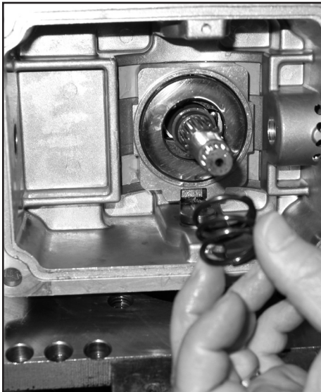
Lift off central spring
